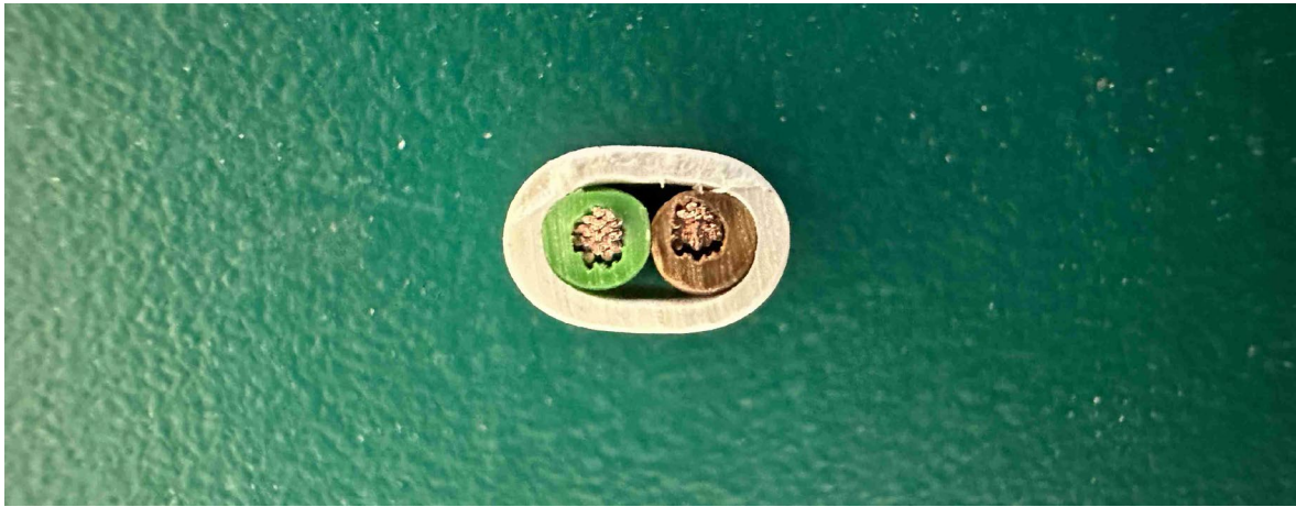
Cold Lead Cross Section
