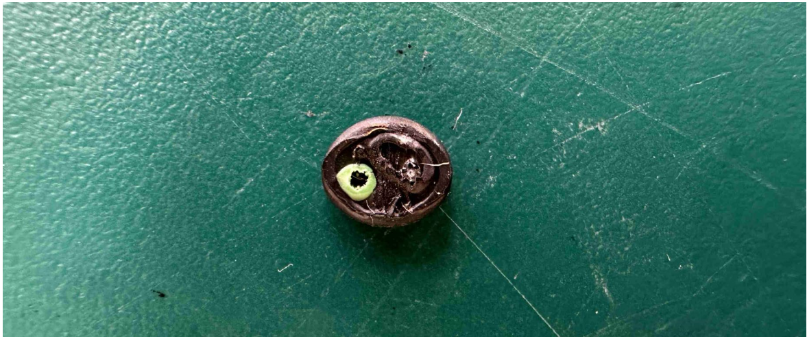
Splice Cross Section
